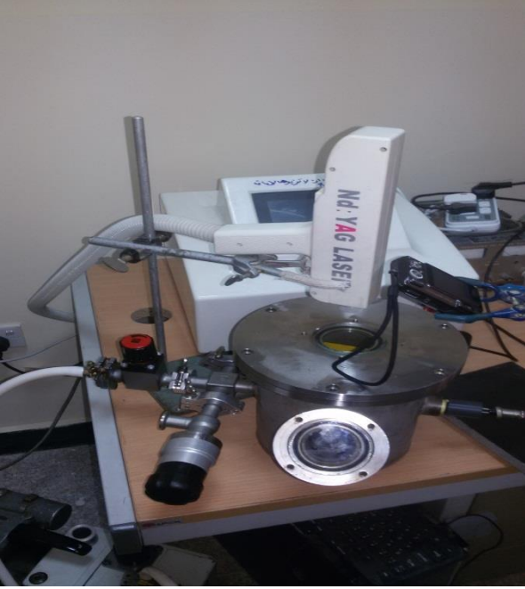
Fig. 3 Experiment set-up used to study the ZnO nanomaterial as a disc.
